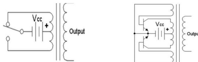
Gambar 1. (a) *Simple inverter push pull* (b) *Auto-Switching inverter push pull*
